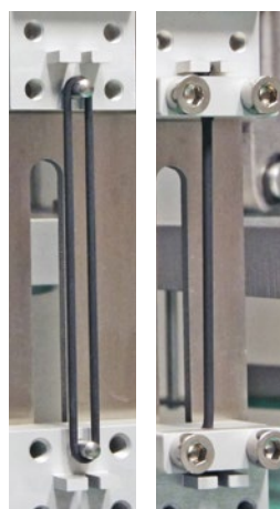
The ET 01.03 grips for O-rings (both whole and cut) are optional for the TR tester.
