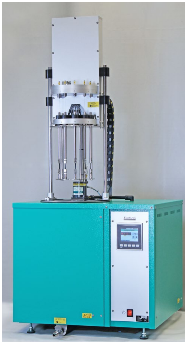
Automatic cooling with liquid nitrogen, ET 01.02.
